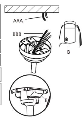
Receiver (B) correctly positioned in the mounting bracket.
